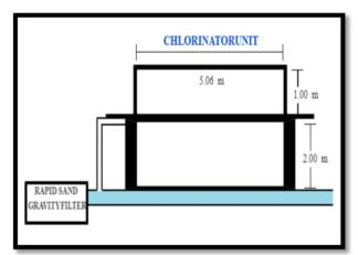
Required for months (n): 6 Unit Height of tank (H): 1 m Height of platform from top level of rapid sand gravity filter: 2 m Density of liquid chlorine (d): 1562.5 kg/m<sup>3</sup>
