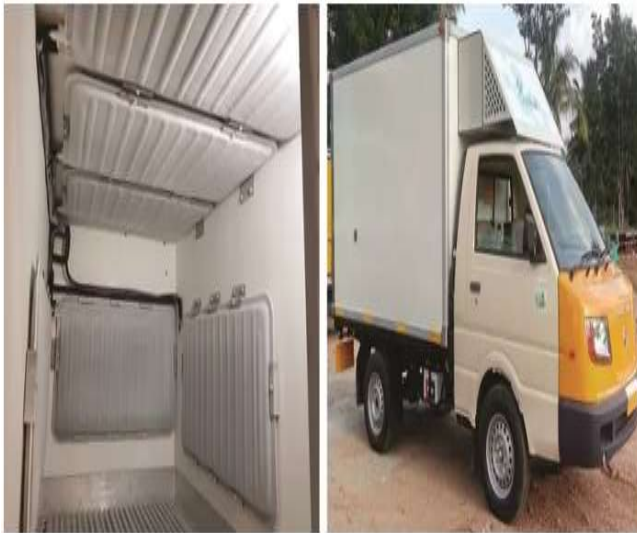
Figure 9: PCM Filled Thermo-tab Active Plates in a Reefer Truck
