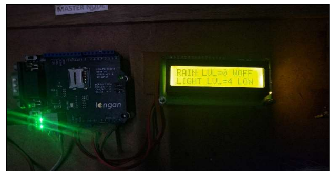
Fig -6: Rain Detection and Smart Lighting results on setup
