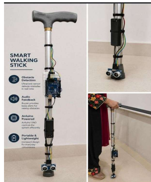
Fig. 3. Real time implementation and experimental setup of the Smart Blind Assistance Stick
