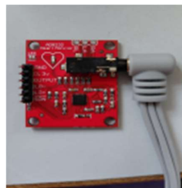
Figure 4: AD8232 ECG Front-End Module and Its Oscilloscope Output
