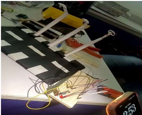
Fig. 3. Real when sensors detect light, the street light turns OFF
