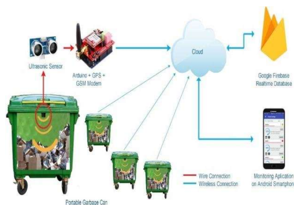
Fig. 3. Smart-bin with sensors (ultrasonic / weight / gas)
