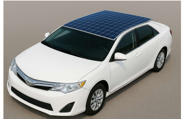
Fig 1: Car with solar panel mounted
