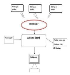
The RFID reader will sends this information to the Arduino Board for further process Arduino performs various operations on the information received by RFID reader by reading RFID tag attached to the product With the help of Arduino, LCD Display will show the name and total cost of the product. If customer wants to remove any any product from list of the purchased product which is already in cart, then customer can remove product.
