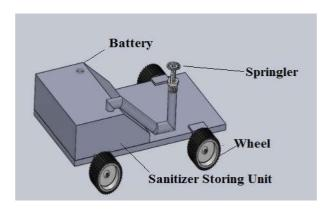
The sanitizer tank is made up of poly ethylene material with capacity of 3 litres.
