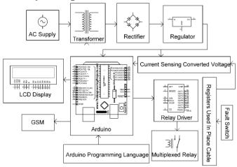
This project deals with Line to Ground fault. Our intention is to find the distance at which fault has occurred. For this we need to first find the resistance of the cable because we know the direct proportionality between the resistance and length.
